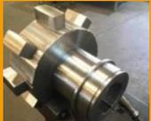
Rejoicing in the difficult, as we do – here is an above average gear replacement job in the workshop - note the tapers running in two directions on each tooth!
